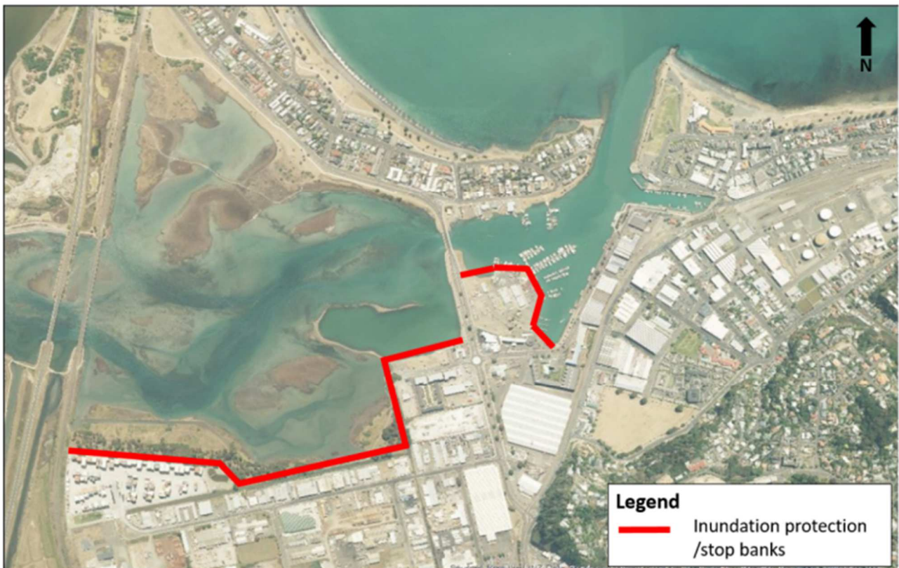
Figure 1-1: Layout of the preferred pathway for the Pandora Unit selected in the stage 3 of the strategy (Bendall, 2018).
